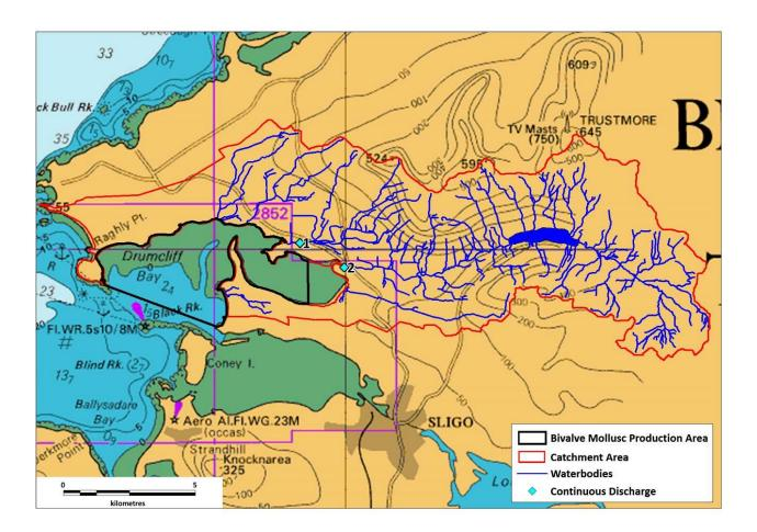
Figure 3.6: Continuous Discharges associated with the Wastewater Treatment Works within the Drumcliff Bay Catchment Area (Source: The EPA, 2019a).
