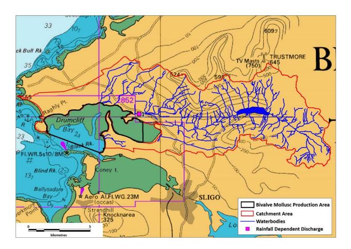
Figure 3.7: Rainfall Dependent Discharges associated with the Wastewater Treatment Works within the Drumcliff Bay Catchment Area (Source: The EPA, 2019a).
